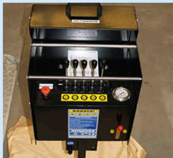
Operator's stand console outside the base
